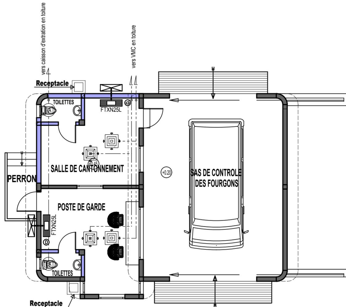
**PLAN DE CLIMATISATION VENTILATION ET VMC**
